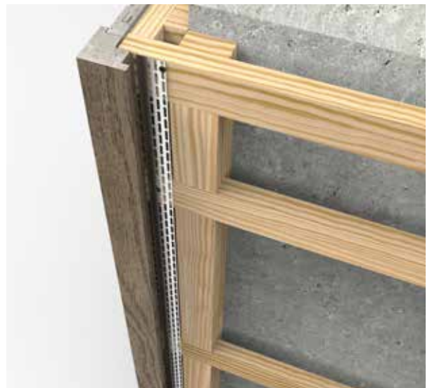
Fig. 8 - External corner detail
