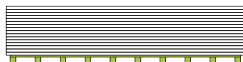
Ensure boards are on a flat surface or bearers max. 400mm apart
